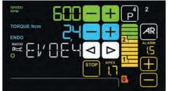
**Endodontics.** During endodontic work the colour LCD control panel displays key data to give the dentist full control over treatment. Everything needed for endodontic treatment is on the dentist's module.
